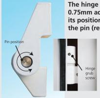
The hinge pin and polymer hinge bearing are both acentric and allow for +/-0.75mm adjustment each to the hinge position. The dot on the top of the pin shows its position and this can be adjusted with an allen key inserted into the bottom of the pin (release the grub screw in the hinge to allow adjustment).
